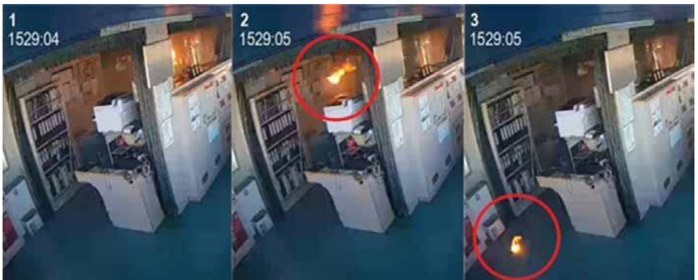
Photos from the bridge closed-circuit camera showing (1) a second explosion occurs, (2) an object is propelled on fire into the air (circled), and (3) the object, still on fire, landing on the floor. (Source: Stalwart Management Ltd and NTSB marine accident report MIR-23-23)
